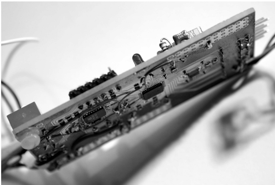
Figure 6.16: Photo of the prototype, the size of the printed circuit board is 7 * 5 cm.
